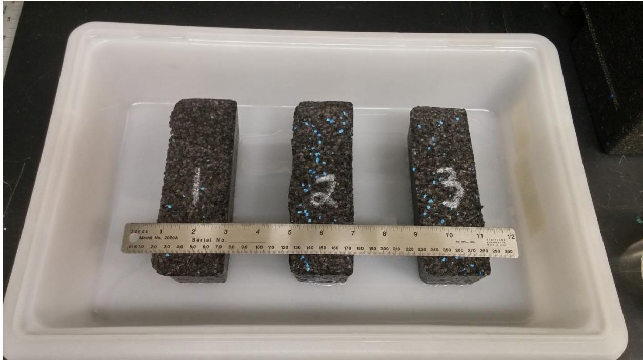
Figure 5. Water Absorption test showing EPP film finish samples prior to filling bath with tap water.
