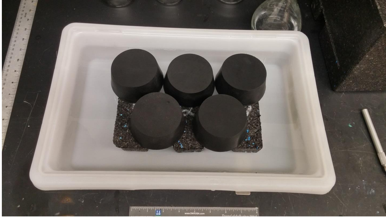
Figure 6. Water Absorption test EPP film finish samples with rubber stoppers weighing down samples to prevent floating.
